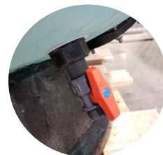
• 3 / 4 " water drain and sand drain
